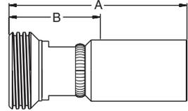
**MATERIAL** Nipple zinc plated high strength special steel, shell stainless steel (AISI 316), other materials on request.
