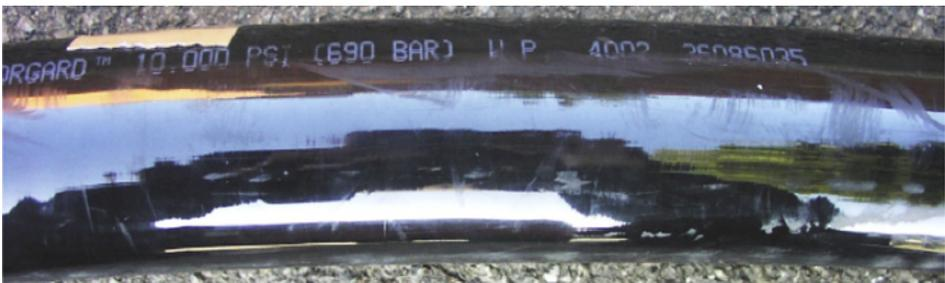
Figure. Photograph of hose cover after the N<sub>2</sub> pressure test
