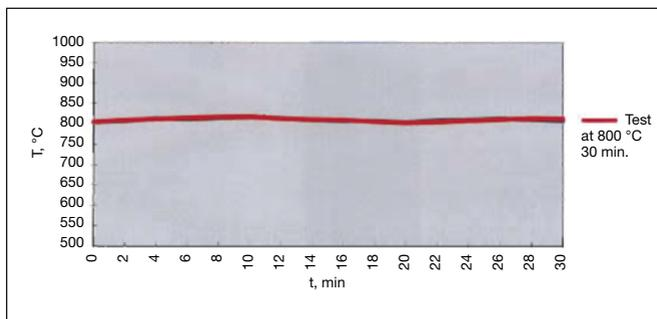
The temperature of the test medium in front of test specimen was 80 °C +/- 2 °C, being the medium behind test specimen 85 °C +/- 2 °C. The flame temperature was 800 °C +/- 50 °C, with actual test duration of 30 min. The measurement records showed satisfactory results.
