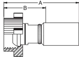
**MATERIAL** Nipple zinc plated high strength special steel, shell stainless steel (AISI 316), other materials on request.
