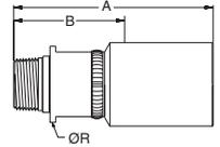
**MATERIAL** Nipple zinc plated high strength special steel, shell stainless steel (AISI 316), other materials on request.
